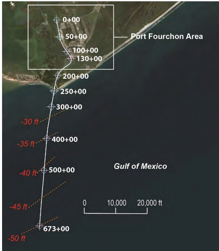
Figure 6: Map diagram of the channel stationing referenced by this study and represents the typical stationing used on previous Port Fourchon projects.
