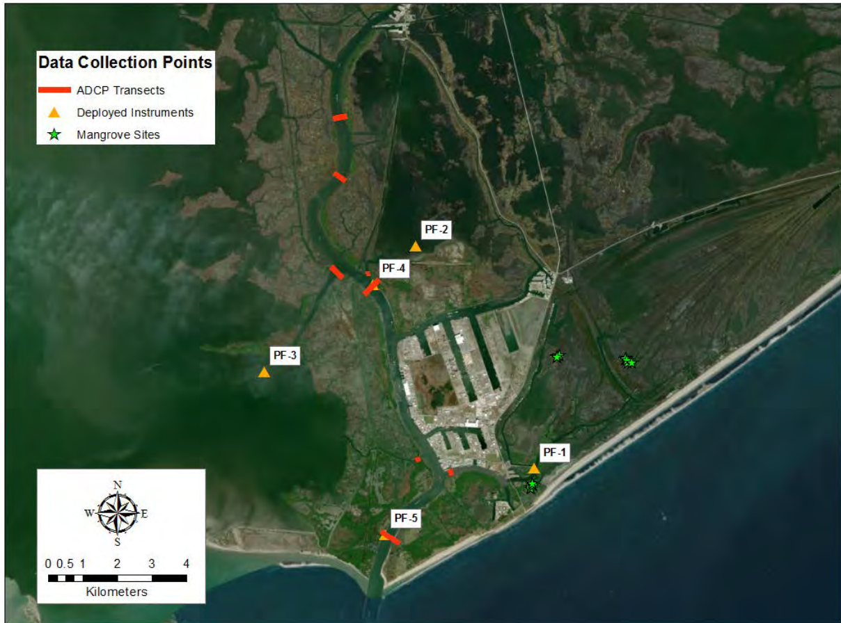
Figure 1. Lower Bayou Lafourche, Port Fourchon, and the Caminada Headland are shown above along with red lines that indicate locations of transects where vessel based ADCP measurements were taken to characterize and quantify flow in the channel. Orange triangles indicate sites where multiparameter water quality sondes are deployed to measure water level, sediment concentration, salinity, and water temperature.
