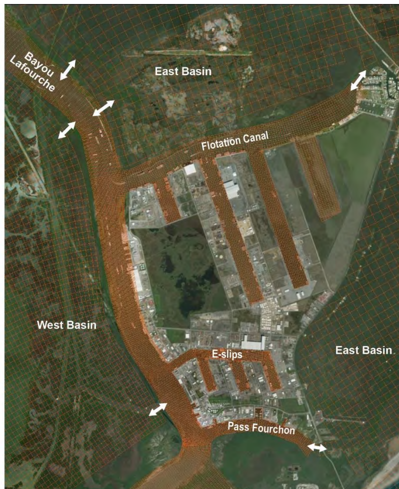
Figure 4: Map diagram of the hydrologic connections between Bayou Lafourche and the proximal basins in the Port Fourchon area. The connections are identified by double-arrow lines.
