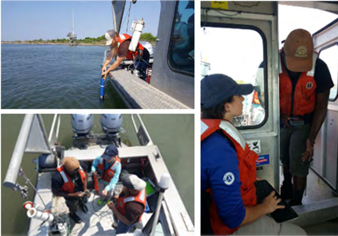
Figure 2. Nicholls State students in action. David Bird, top left, takes a spot reading of water salinity, temperature, and turbidity with a YSI multiparameter sonde. Bottom left, Andrea Jarebek shows David Bird and Olijuwan Jimoh how to set up a data collector to take a water quality measurement with the YSI. On the right frame, Olijuwan Jimoh shares the reading from the data logger with Kellyn LaCoeur-Conant as she updates the on-board GIS map on the shipboard computer.
